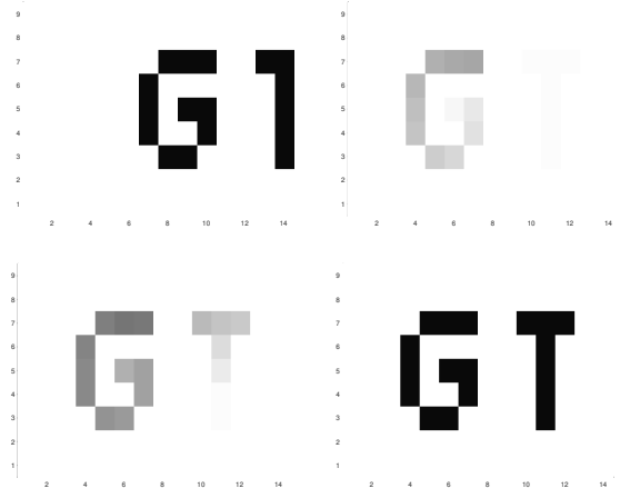
Fig. 2: Snapshots of an animation that illustrates the simultaneous control of oscillators: each oscillator is a pixel. Time instances of these 4 snapshots: 0:02, 0:06, 0:07, 0:10.
