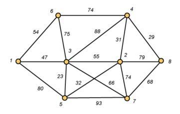
Problem The vertices represent 8 regional data centers which need to be connected with high-speed data lines. Feasibility studies show that the links illustrated above are possible, and the cost in millions of dollars is shown next to the link. Which links should be constructed to enable full communication (with relays allowed) and keep the total cost minimal?
