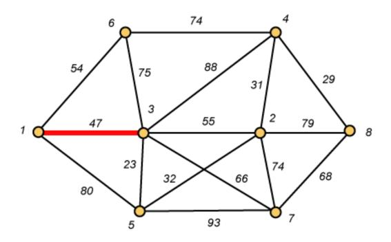
Remark In this example, we take vertex 1 as the "root" and start with the trivial tree consisting of just the root. We illustrate the first step after the initialization step.
