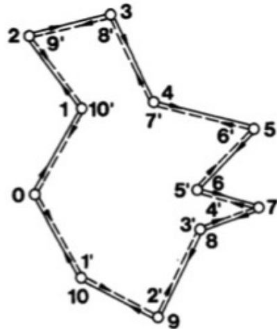
Fig. 2.5. Diffusion path of the conduction electron in the disordered system. The electron propagates in both directions (full and dashed lines). In the case of quantum diffusion the probability to return to the origin is twice as great as in classical diffusion since the amplitudes add coherently.
