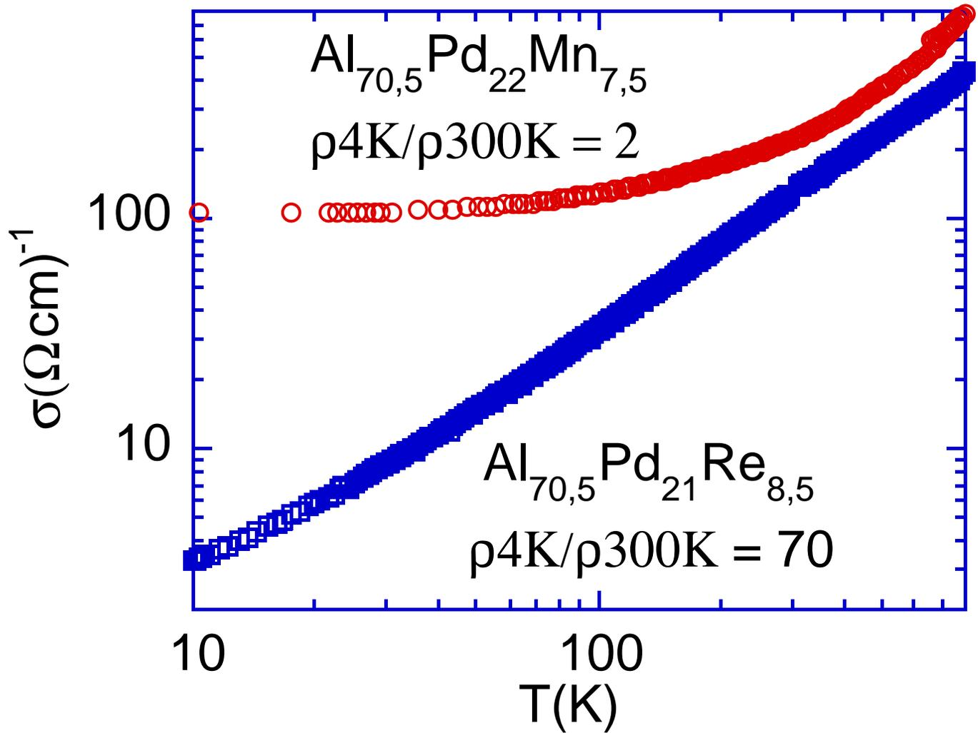
Conductivity of Quasicrystals vs Temperature
