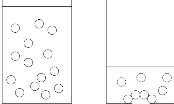
FIG. 1.1. *Suspension in a container. The left-hand image shows the container filled with the suspension before the opening is made. The right-hand image shows the system at the moment the opening clogs.*
