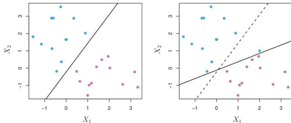
**FIGURE 9.5.** Left: Two classes of observations are shown in blue and in purple, along with the maximal margin hyperplane. Right: An additional blue observation has been added, leading to a dramatic shift in the maximal margin hyperplane shown as a solid line. The dashed line indicates the maximal margin hyperplane that was obtained in the absence of this additional point.
