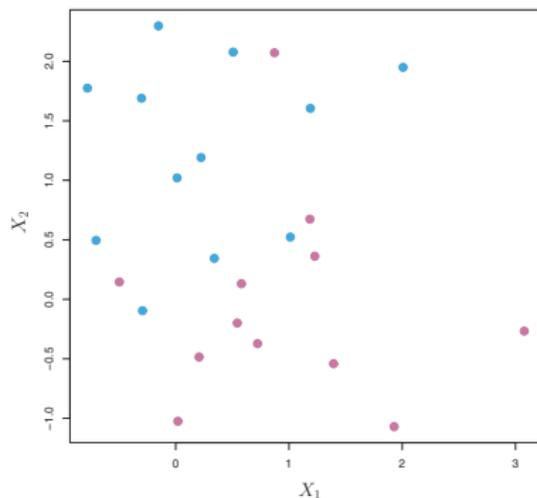
**FIGURE 9.4.** *There are two classes of observations, shown in blue and in purple. In this case, the two classes are not separable by a hyperplane, and so the maximal margin classifier cannot be used.*
