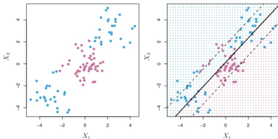
**FIGURE 9.8.** Left: The observations fall into two classes, with a non-linear boundary between them. Right: The support vector classifier seeks a linear boundary, and consequently performs very poorly.
