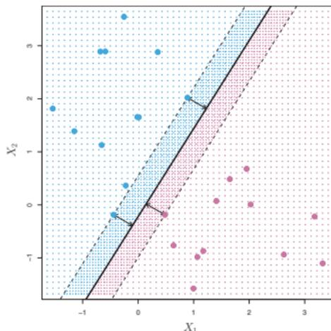
**FIGURE 9.3.** There are two classes of observations, shown in blue and in purple. The maximal margin hyperplane is shown as a solid line. The margin is the distance from the solid line to either of the dashed lines. The two blue points and the purple point that lie on the dashed lines are the support vectors, and the distance from those points to the hyperplane is indicated by arrows. The purple and blue grid indicates the decision rule made by a classifier based on this separating hyperplane.
