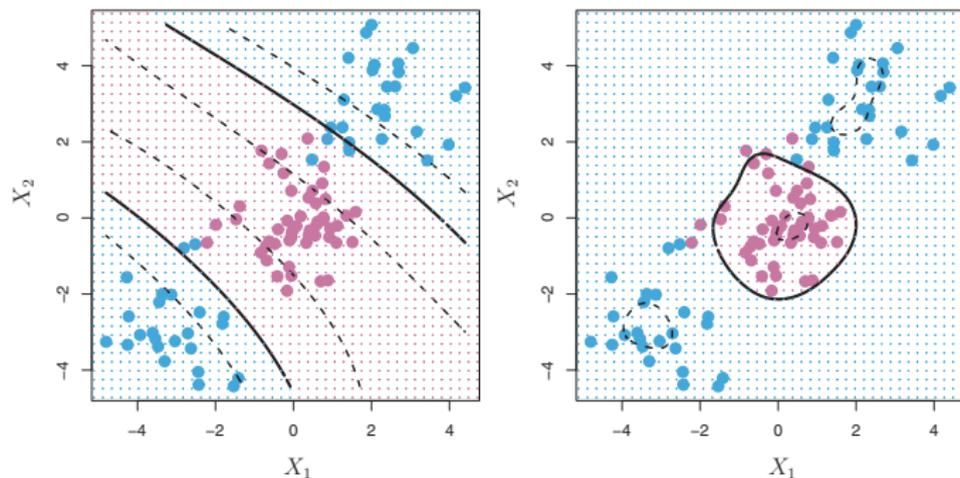
**FIGURE 9.9.** Left: An SVM with a polynomial kernel of degree 3 is applied to the non-linear data from Figure 9.8, resulting in a far more appropriate decision rule. Right: An SVM with a radial kernel is applied. In this example, either kernel is capable of capturing the decision boundary.
