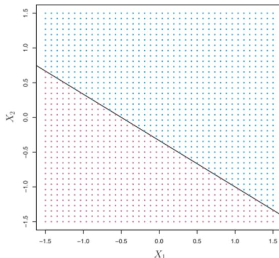
**FIGURE 9.1.** The hyperplane  $1 + 2X_1 + 3X_2 = 0$  is shown. The blue region is the set of points for which  $1 + 2X_1 + 3X_2 > 0$ , and the purple region is the set of points for which  $1 + 2X_1 + 3X_2 < 0$ .
