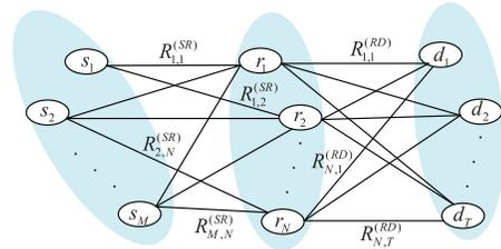
Fig. 1. A relay aided system with  $M$  sources,  $N$  relays, and  $T$  destinations.
